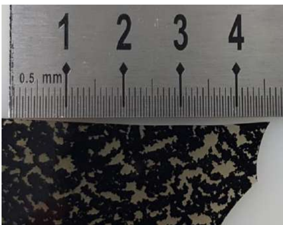
Fig. 3. Example of extreme visual CNT agglomeration in epoxy resin at 0.5% wt.
